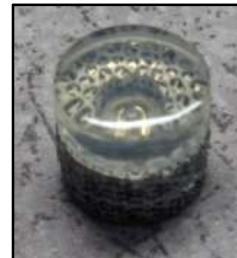
A 10 mm SynACART osteochondral implant. The polycarbonate urethane articulating surface is backed by an OsteoSync Ti bone ingrowth region.
